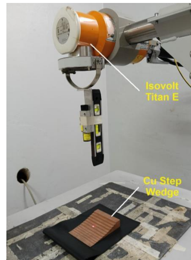
Figure 2. Experimental setup for SNR measurement using copper step wedge
