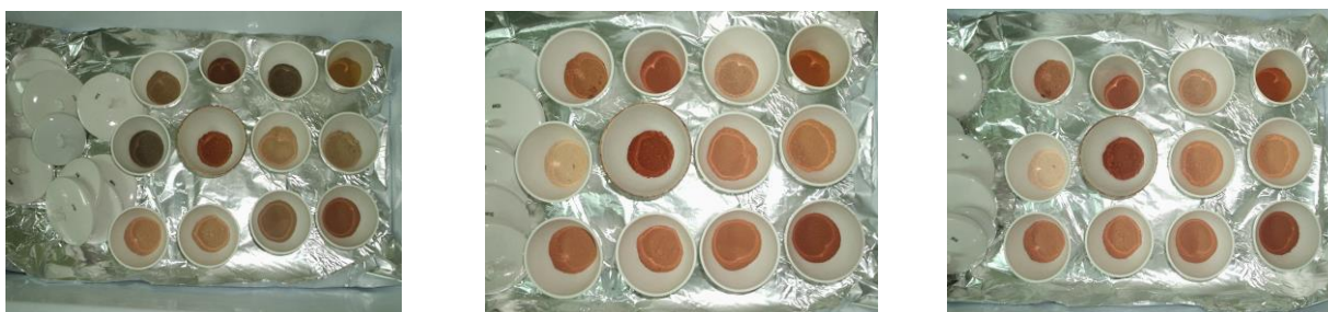
Figure 3a. LOI (from left to right) at 105 °C, 550 °C and 1000 °C)
