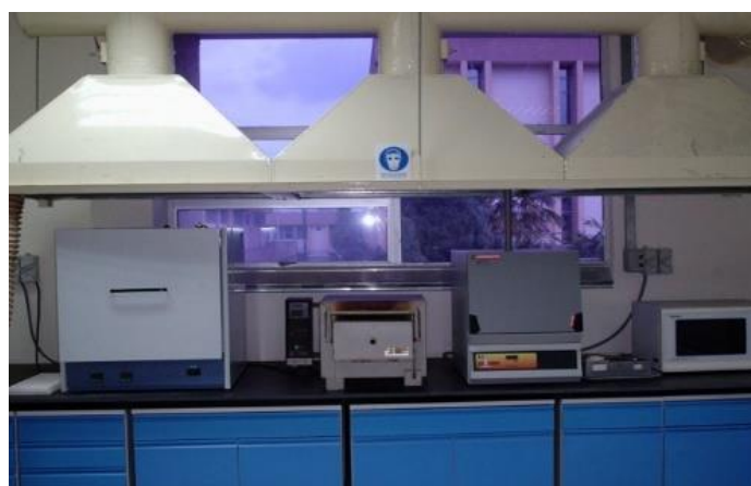
Figure 3b. Furnace for LOI
