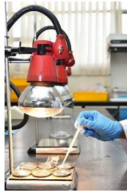
Figure 1. Sample drying under an infrared lamp
