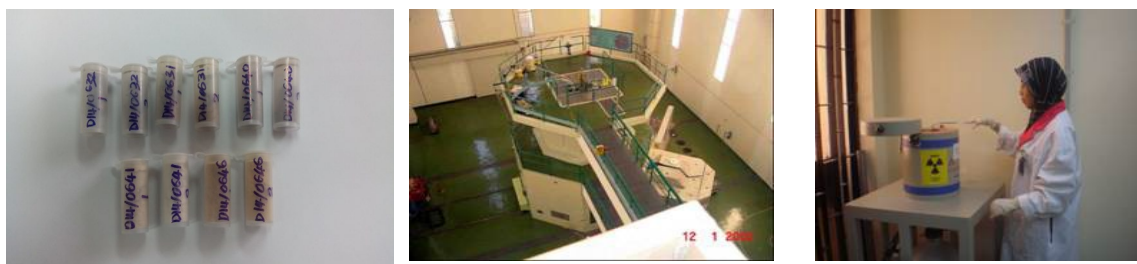
Figure 4. NAA metal analysis (from left to right): Samples, neutron irradiation, gamma counting
