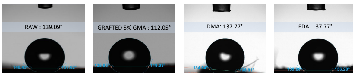
Figure 7(a). Contact angle for raw, grafted and modified industrial PE filter cartridge with 5 wt% of GMA
