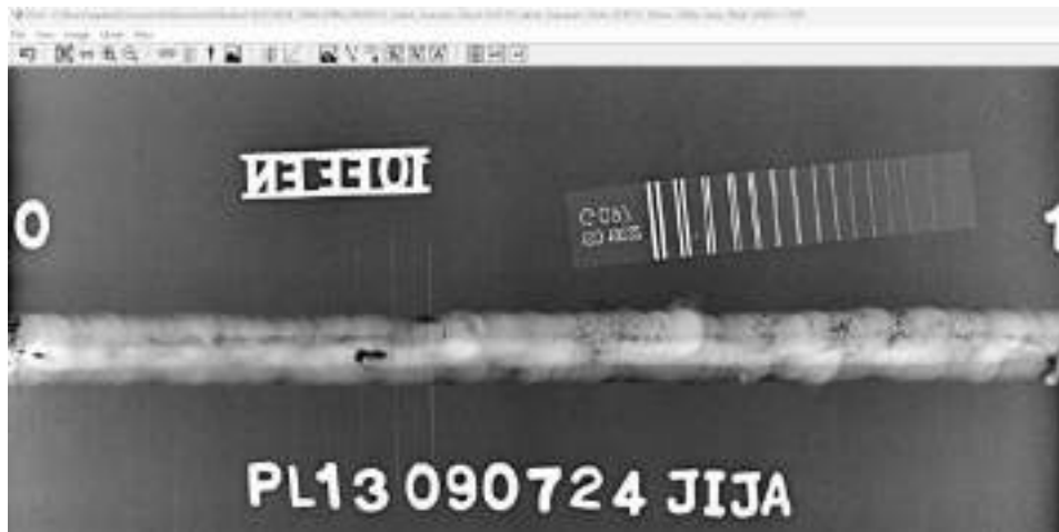
Figure 8. Radiograph image for welded plate using imaging plate for 140 kV beam energy
