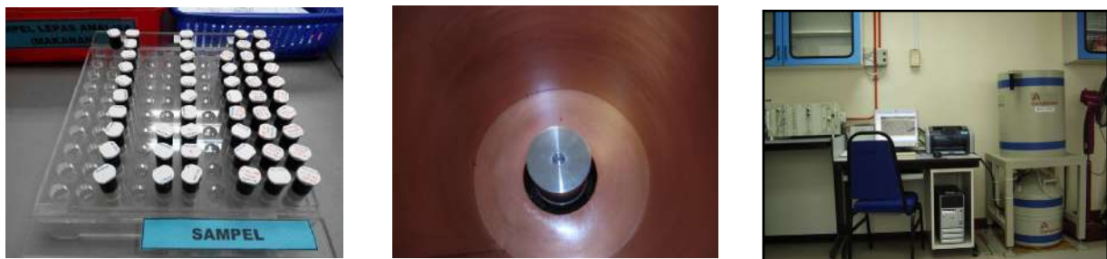
Figure 3. Radioactivity measurement (from left to right): samples, well detector, gamma spectrometry system.
