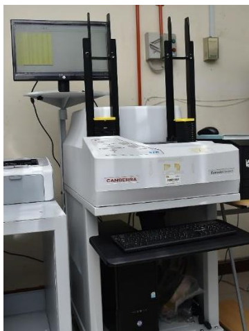
Figure 1. Low background gross alpha beta counting system
