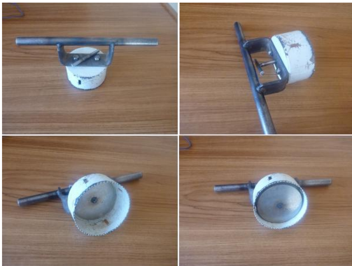
Figure 2: A metal scraper hand tool for CSSI sampling
