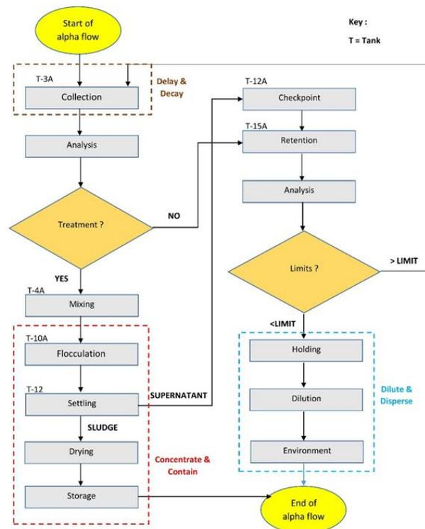
Fig. 1. Flowchart for Treatment of Aqueous Liquid Waste containing Alpha Emitters at Low Level Effluent Treatment Plant (LLETP), Nuclear Malaysia.
