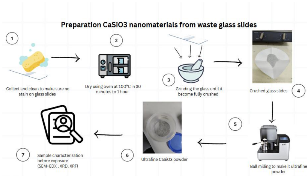
Figure 1: Preparation of CaSiO 3 Glass Nanomaterials before exposure
