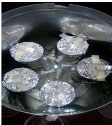
Fig. 1. Culture plates were wrapped with aluminium foil and irradiated in the gamma cell.
