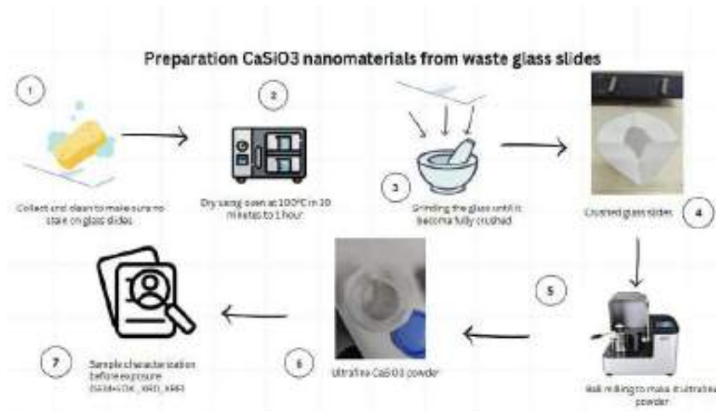
Figure 1: Preparation of CaSiO 3 Glass Nanomaterials before exposure
