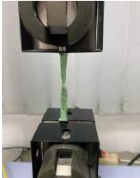
Figure 1: Tensile strength test using Universal Tensile Machine (UTM)
