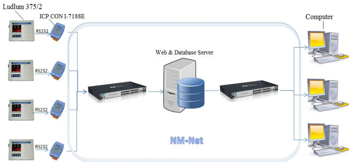
Figure 1: Block diagram of the radiation area monitoring system
