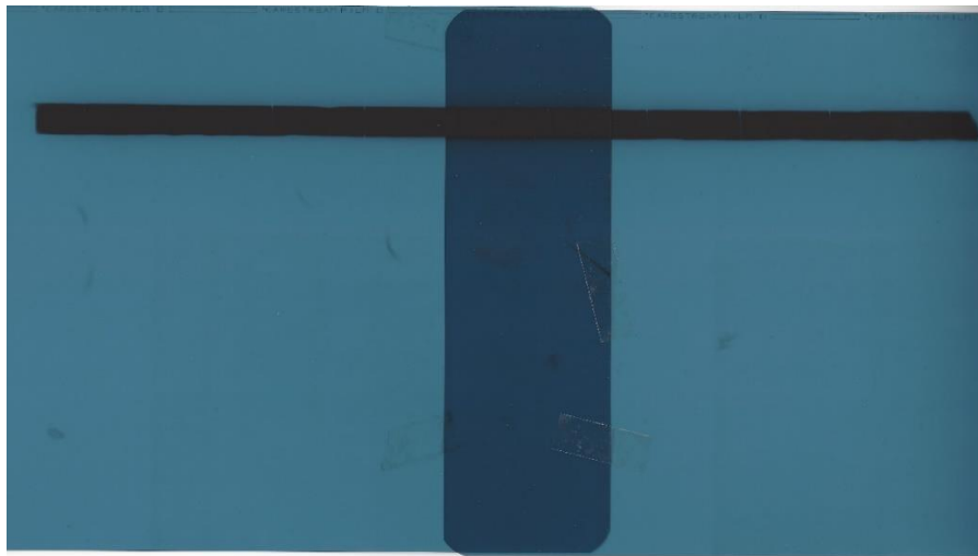
Figure 9: X-ray fan beam image on two MXG films put on rotation table right at center of rotation (COR). The images are overlapped together by using 7 needles as reference position for image alignment
