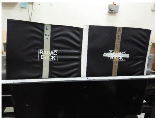
Figure 3: MXG films covered in X-ray film holders in front of LAD
