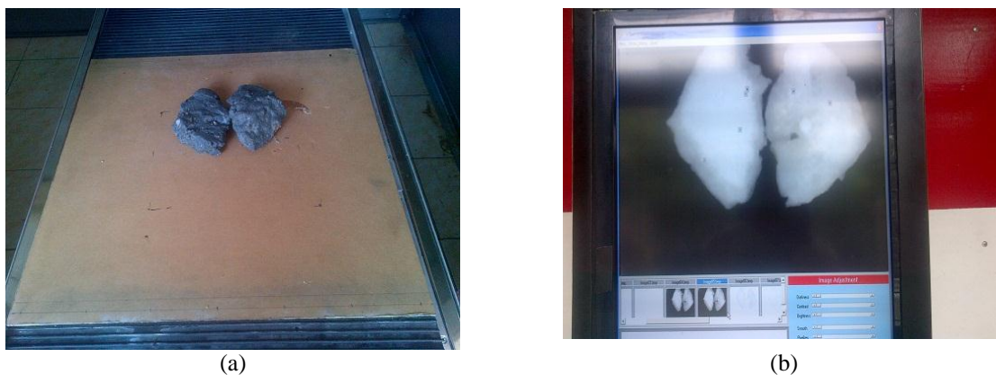
Figure 1: A radioscopy-based digital radioscopy system at the Gadjah Mada University. (a) Object on conveyer, (b) Display monitor and control panel
