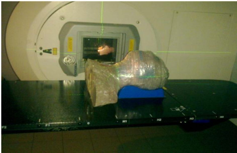
Fig. 4: Anatomical Perspex head and neck phantom during 3D-CRT treatment
