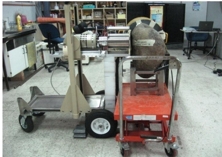
Figure 6: In-situ irradiation of samples at Malaysian Nuclear Agency
