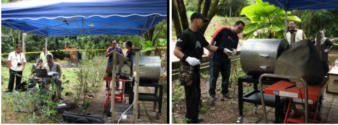
Figure 7: The process for in-situ irradiation of dolerite rock samples in Hulu Sungai Lawit, Tasik Kenyir
